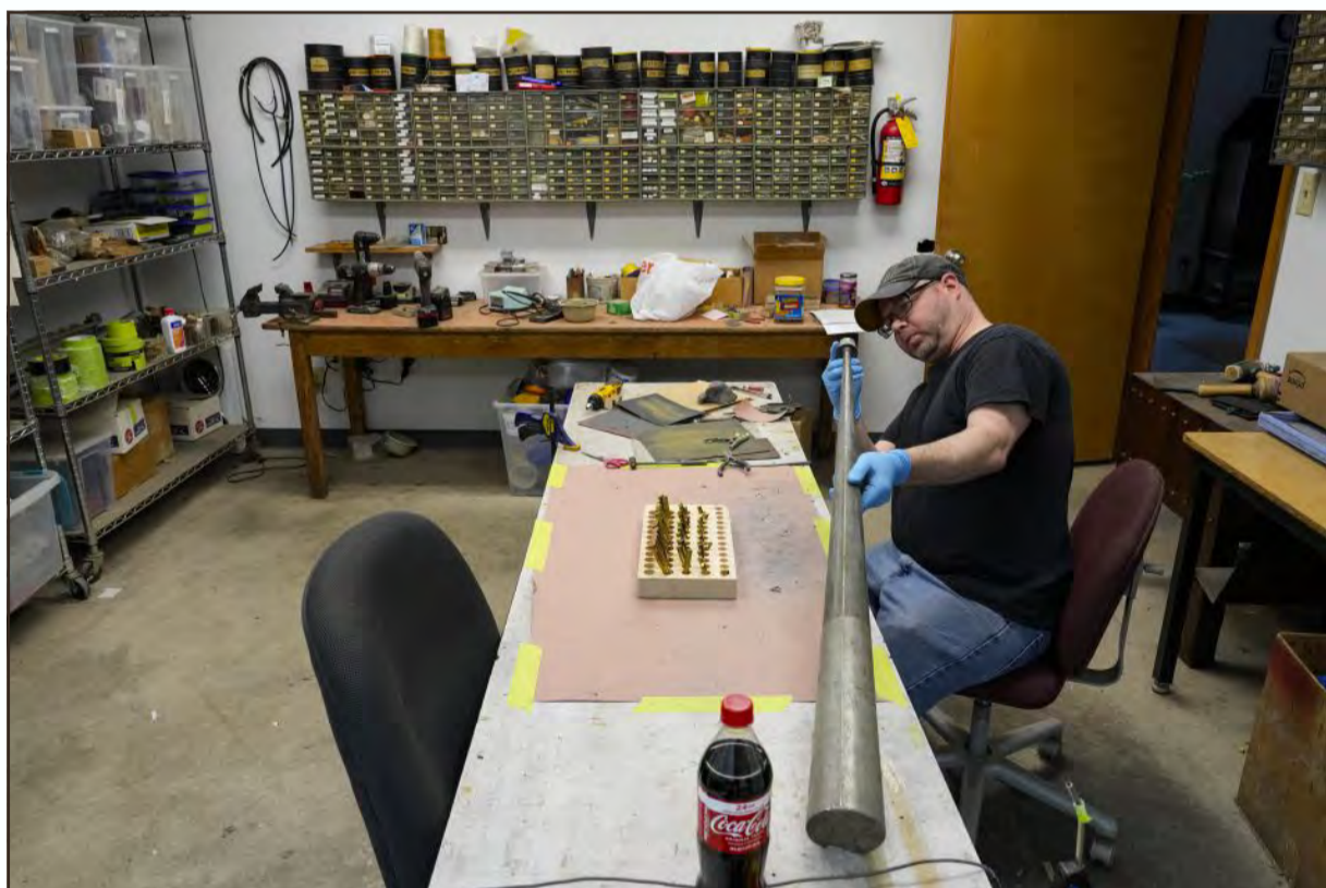
Nimmo removes the reed from one of the hundreds of pipes that are part of the Barton Opus 234 theater organ.
