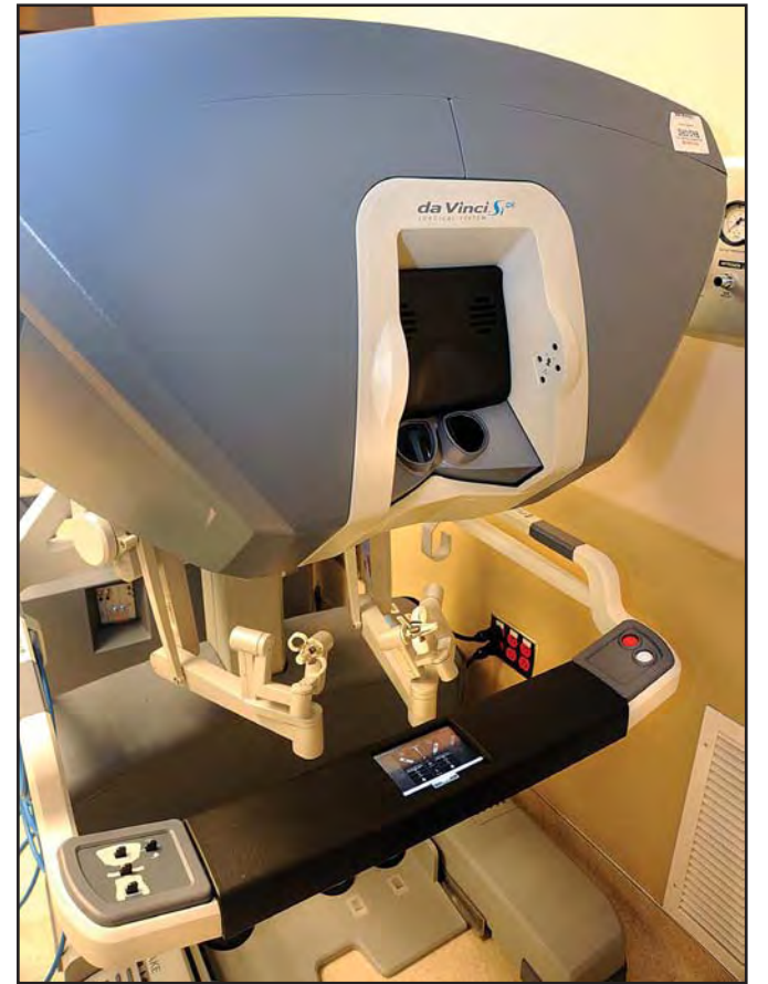
The console where surgeons sit (above) to control the system can be adjusted for comfort, allowing a surgeon to work without being fatigued. A monitor (below) shows a surgeon tying a suture using the da Vinci Robotic System.
